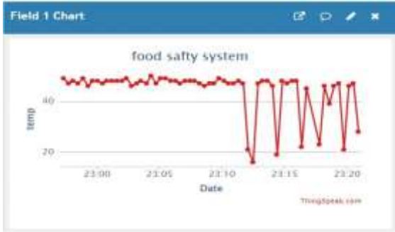
Fig 9: Temperature sensor results
